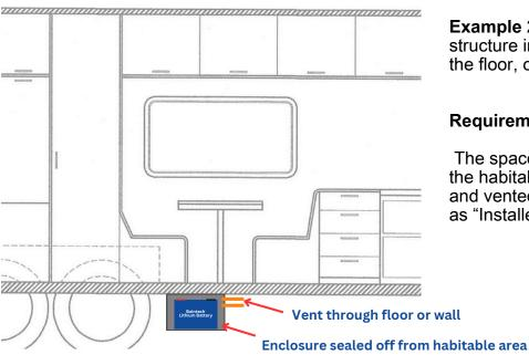
**Example 2**: Installed outside the structure in an enclosure, i.e. under the floor, on the drawbar
